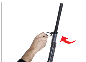
17- Gas chamber nut is fixed.
