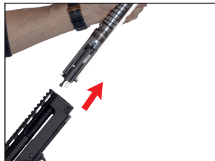
10- Remove bolt barrel assembly.
