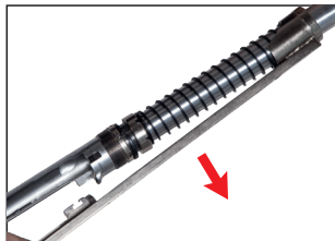
12- Remove bolt, and bolt carrier.
