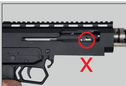
For charging handle placement, hole is not proper.
