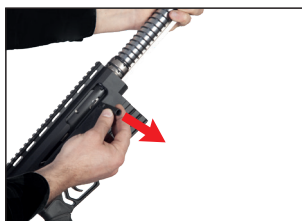
8- Remove charging handle, please make sure that bolt carrier is pulled a bit backside to remove charging handle easily.
