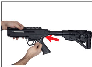
13- Remove upper lower by removing pins.
