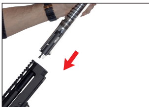
10- Put this assembly inside receiver.
