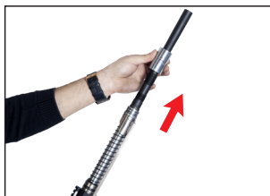
6- Remove gas chamber.
